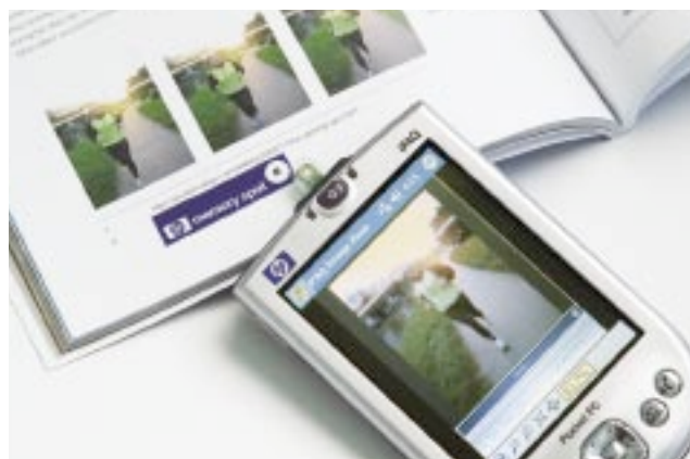
Memory Spot embedded in a book could provide supplemental text, images and video to anyone with a portable reader.
