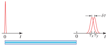
Figure 9.3-7 Differential group delay (DGD) associated with polarization mode dispersion (PMD).
