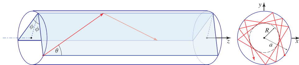
Figure 9.1-2 A skewed ray lies in a plane offset from the fiber axis by a distance R . The ray is identified by the angles \theta and \phi . It follows a helical trajectory confined within a cylindrical shell with inner and outer radii R and a , respectively. The projection of the ray on the transverse plane is a regular polygon that is not necessarily closed.
