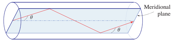
Figure 9.1-1 The trajectory of a meridional ray lies in a plane that passes through the fiber axis. The ray is guided if \theta < \bar{\theta}_c = \cos^{-1}(n_2/n_1) .
