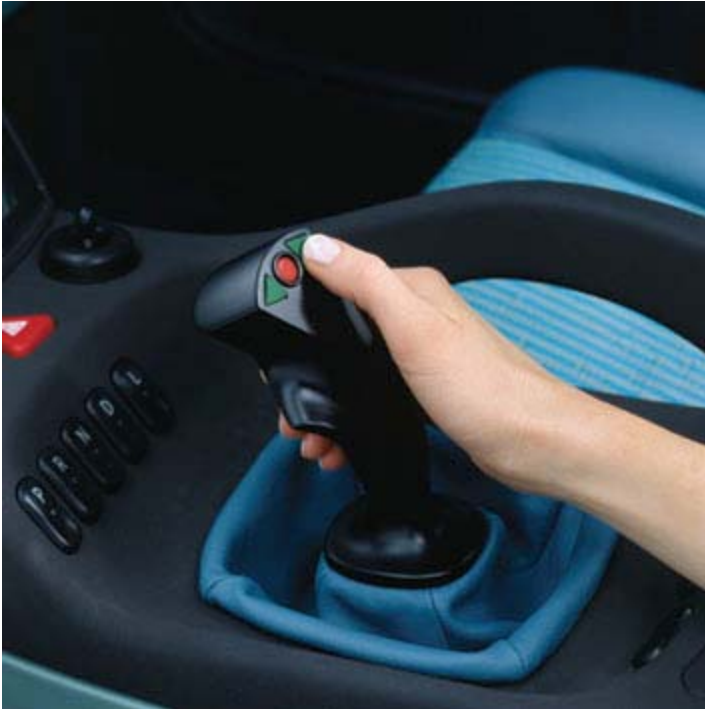
The sidestick, being tested by Mercedes-Benz, is part of a fully computer-controlled car handling system of the possibly near future.
